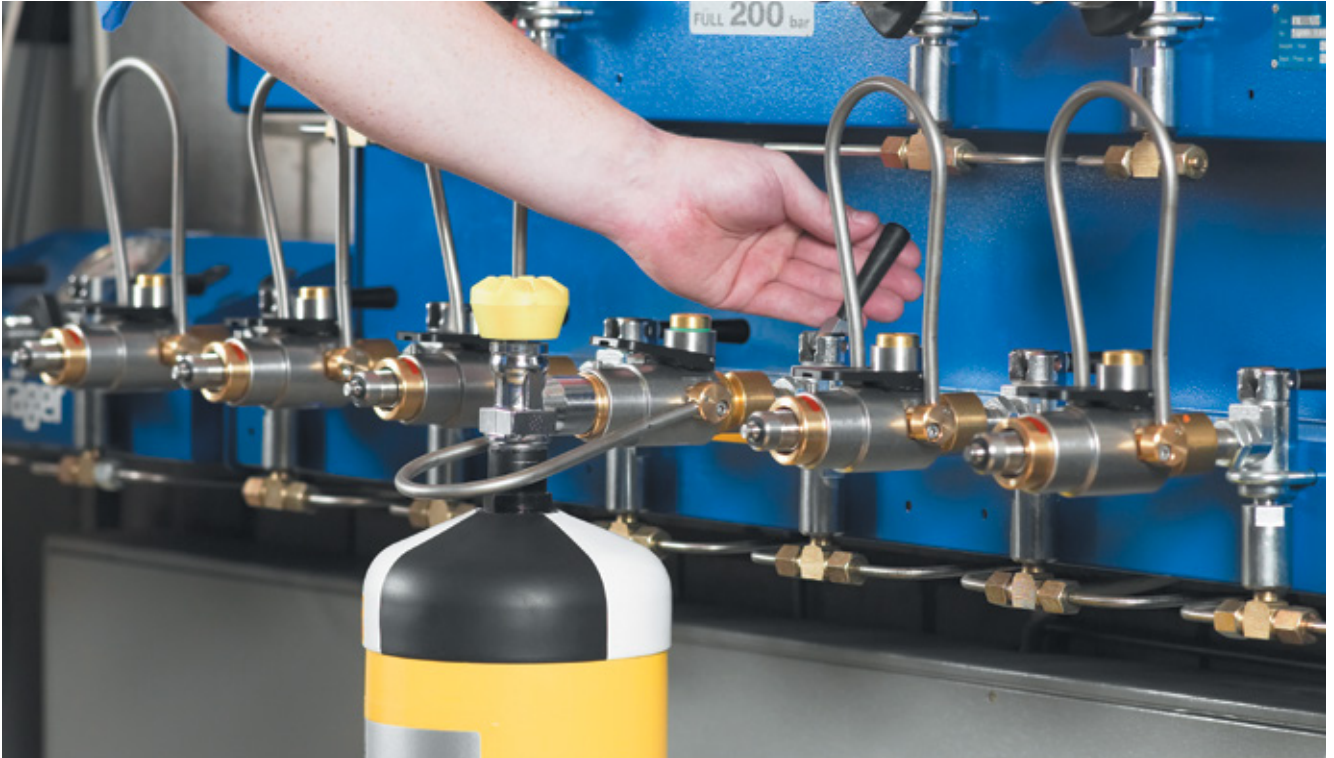
Existing BA cylinder filling rig after it has been upgraded to using the CLICKMATE® TW154
