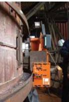
Re-gen head with 'C' plates and wedges positioned
